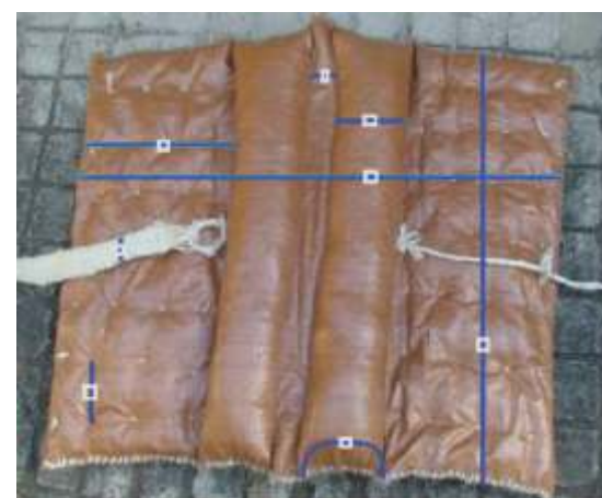
Figure 1. Measurements of the upper side of the packsaddle prototype developed; the upper side is a fertilizer sack, which is waterproof and hence durable
