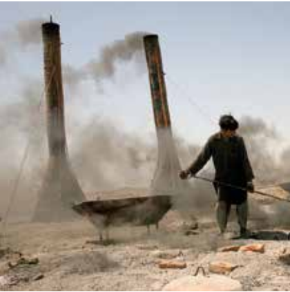
Movable Chimney Bull's Trench Kiln (MCBTK) © 2017 Tomas Munita
